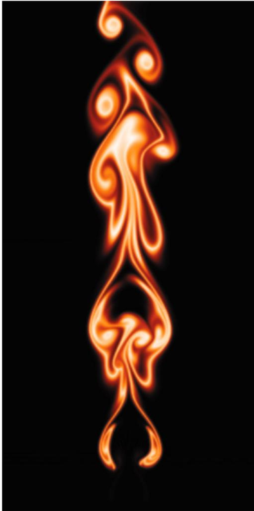
Turbulence enhances combustion thanks to increased mixing:
