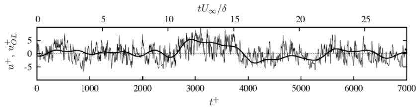
**Fig. 2.** Example of fluctuating signal  $u^+$  at  $z^+ = 15$  and large-scale fluctuating component  $u_{OL}^+$  in the outer layer (thick blank line) at  $z^+ = 330$  measured in a turbulent boundary layer at  $Re_\tau = 7300$ .
