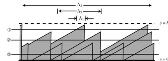
Simplified hairpin-vortex-packet model used to describe the distribution of streamwise kinetic energy among scales. Mean flow is from left-to-right. Hairpin vortex packets of differing scales are indicated as shaded regions.
