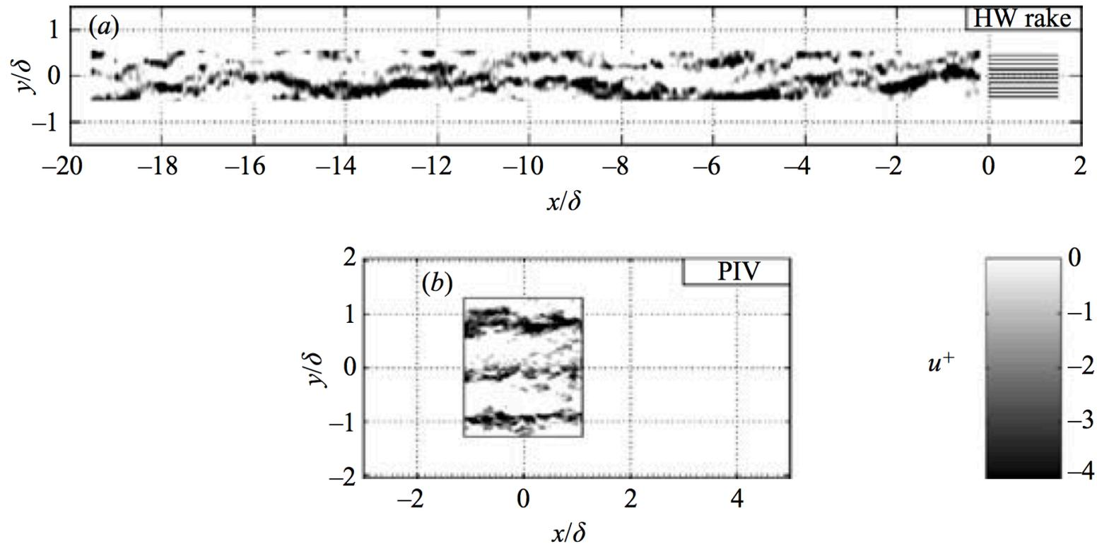
FIGURE 4. (a) Example of rake signal at  $z/\delta = 0.15$  for  $Re_\tau = 14\,380$ . The  $x$ -axis is reconstructed using Taylor's hypothesis and a convection velocity based on the local mean,  $\bar{U} = 15.9 \text{ m s}^{-1}$ . (b) Typical PIV frame for comparison at  $Re_\tau = 1100$ ,  $z/\delta = 0.087$ . Shading shows only negative  $u$  fluctuations (see grey-scale).
