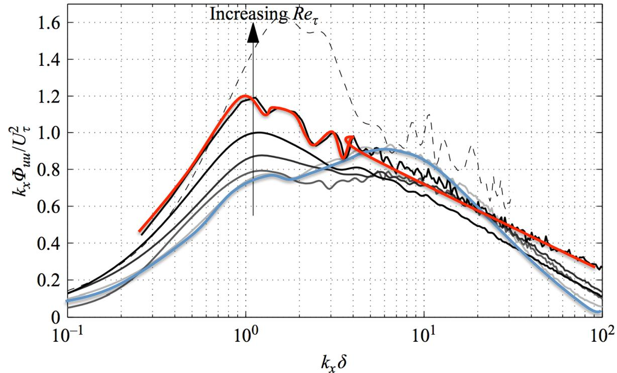
FIGURE 9. Pre-multiplied energy spectra  $k_x \Phi_{uu} / U_\tau^2$  at  $z/\delta = 0.06$  for laboratory hot-wire measurements. Line shading indicates Reynolds number. From lightest to darkest  $Re_\tau = 1010, 1910, 2630, 4110$  and  $7300$ . Dashed line shows sonic anemometer data from SLTEST (Utah 2005) at  $Re_\tau \approx 6.6 \times 10^5, z/\delta = 0.06$ .
