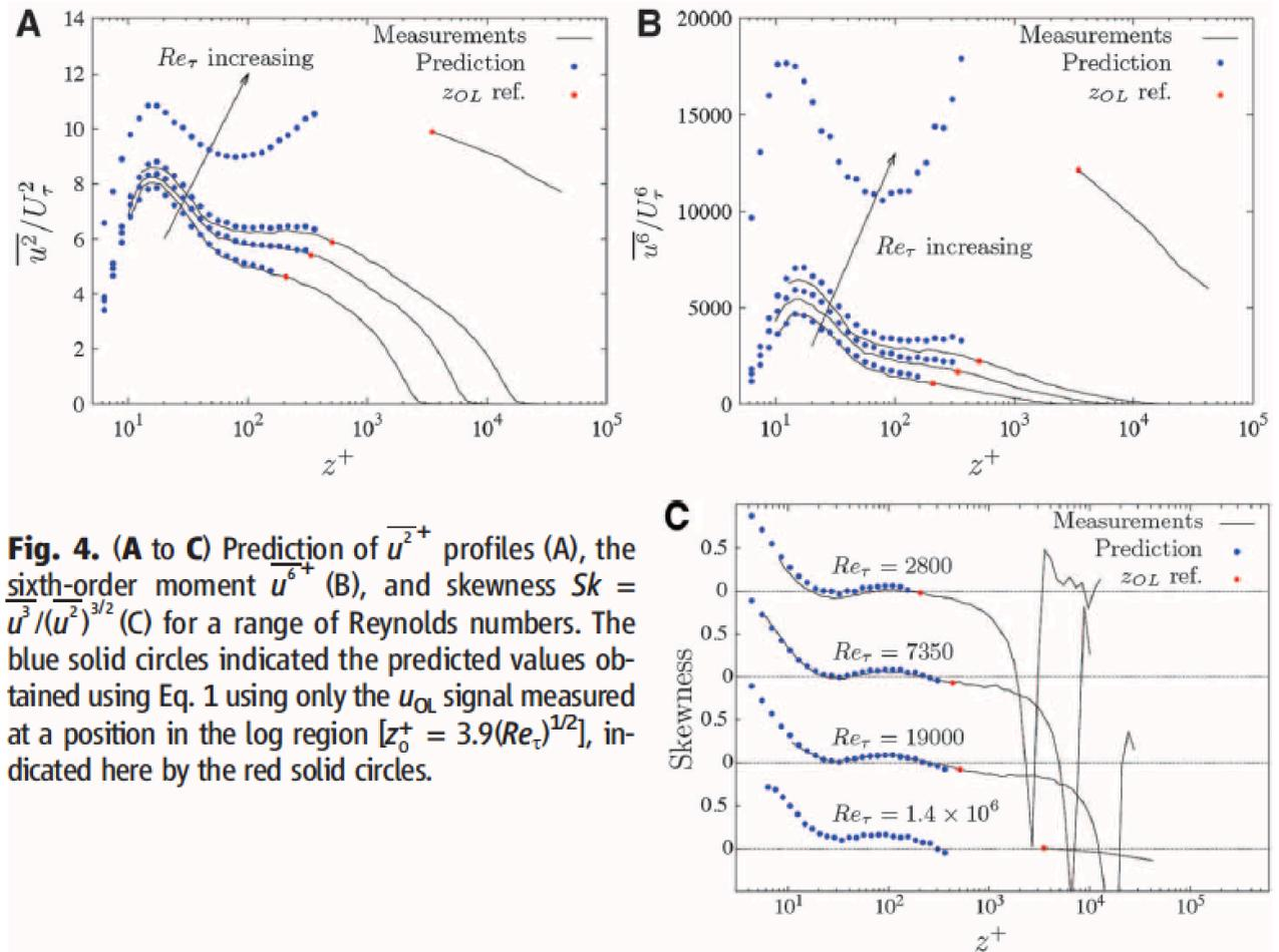
**Fig. 4. (A to C)** Prediction of  $\overline{u^{2+}}$  profiles (A), the sixth-order moment  $\overline{u^{6+}}$  (B), and skewness  $Sk = \overline{u^3}/(\overline{u^2})^{3/2}$  (C) for a range of Reynolds numbers. The blue solid circles indicated the predicted values obtained using Eq. 1 using only the  $u_{OL}$  signal measured at a position in the log region [ $z_0^+ = 3.9(Re_\tau)^{1/2}$ ], indicated here by the red solid circles.
